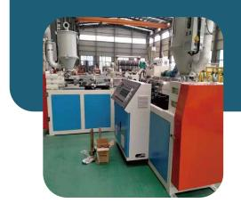
**Range Optional Extruder** for Adhesive Lined **Dual Wall Heat Shrink Tubing**
